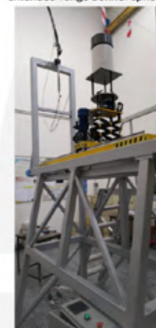
Figure 3. Test of a LUPIN-II monitor at the UPM irradiation bench.
