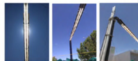
Bottom view of concentrated sunlight over receiver
